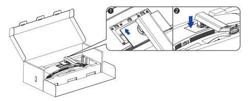
④ Install the Stand-Base to the Stand-Neck and then tighten the thumb screw to secure it.
