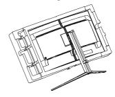
While keeping the release button pressed, tilt the stand and slide it out.
