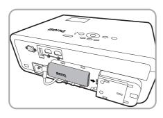
5. Arrange the USB Micro B cable in place below the dongle.
