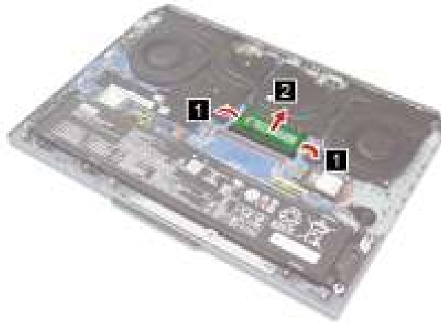
Figure 17. Open the latches and remove the memory module
