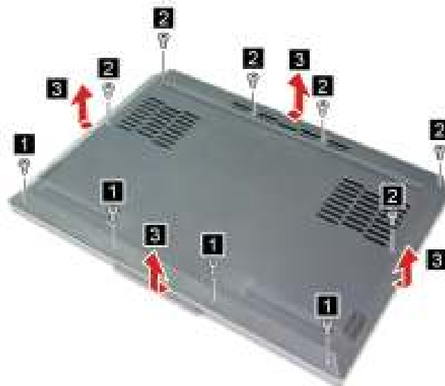
Figure 5. Remove ten screws and the lower case
