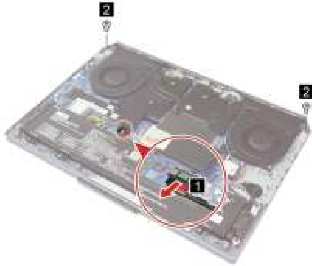
Figure 18. Disconnect the battery pack cable and remove two screws
