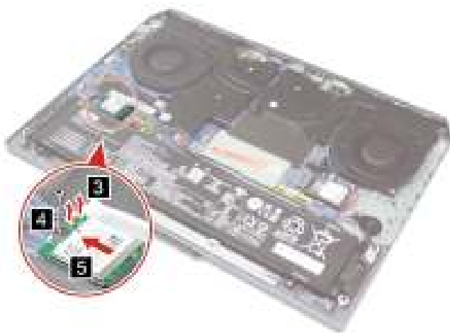
Figure 11. Disconnect the antennas, remove one screw and the Wi-Fi card
