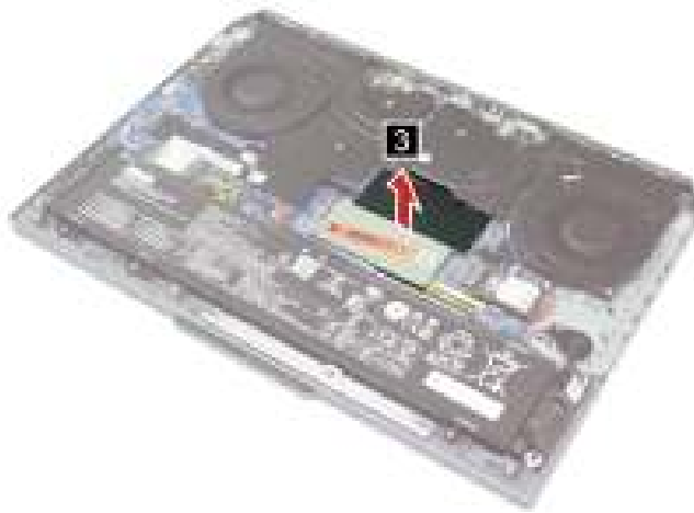
Figure 16. Remove the DIMM shielding
