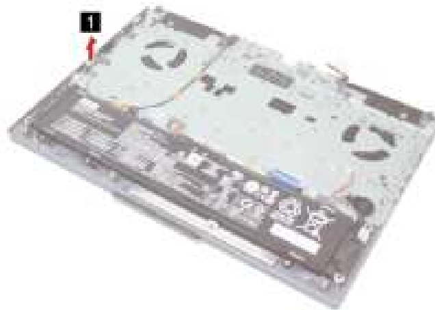
Figure 25. Remove the Type-C bracket
