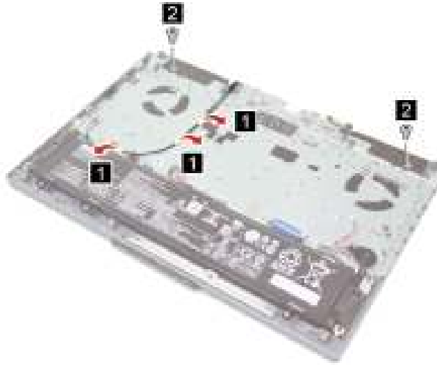
Figure 26. Remove two screws and remove the antennas from the cable guide
