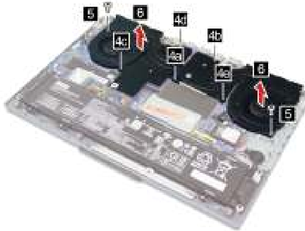
Figure 21. Loosen five heat sink screws, remove two fan screws, and remove the thermal module
