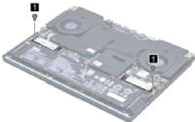
Figure 10. Remove two screws
