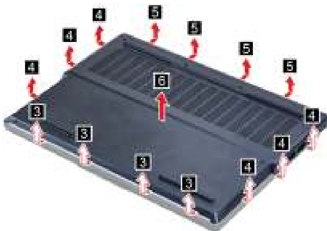
Figure 6. Pry up the latches and remove the lower case
