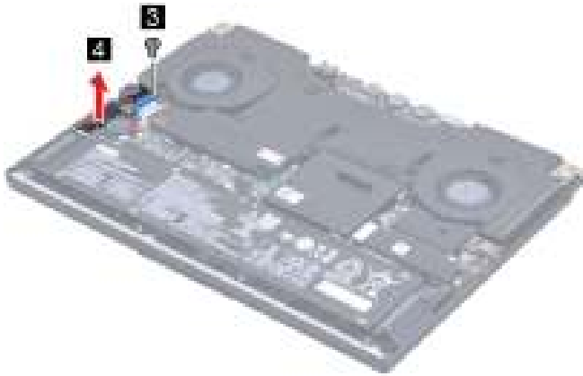
Figure 26. Remove the I/O board
