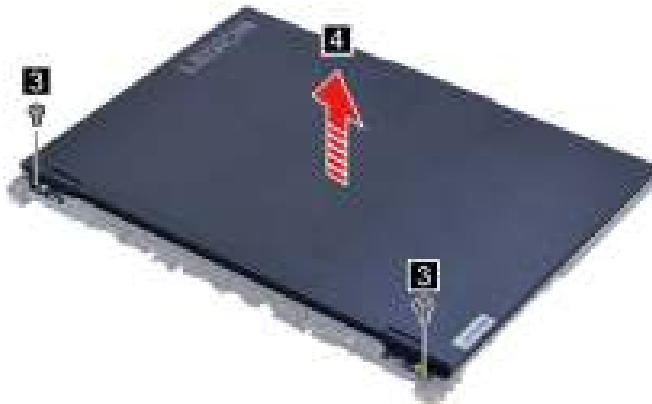
Figure 51. Lift the LCD module
