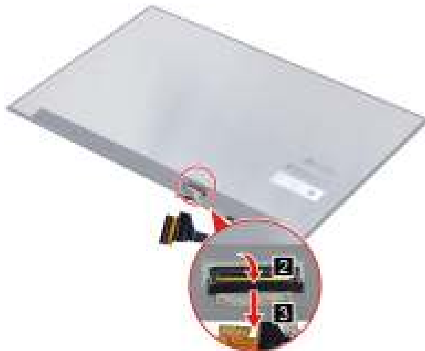
Figure 63. Remove the EDP cable
