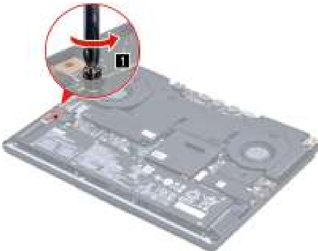
Figure 12. Remove the SSD stand off
