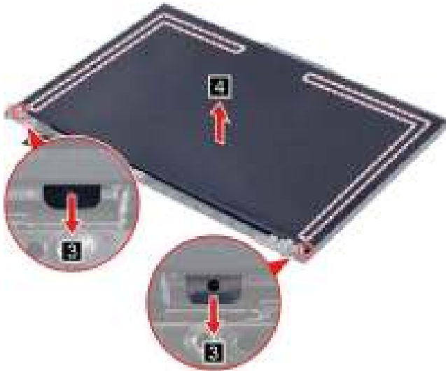
Figure 61. Remove the LCD panel
