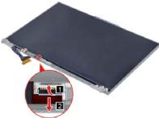
Figure 60. Disconnect the EDP cable from the sensor board and release the EDP cable
