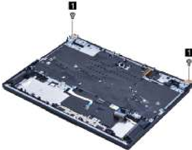
Figure 48. Remove two screws
