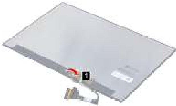
Figure 62. Peel off the tape
