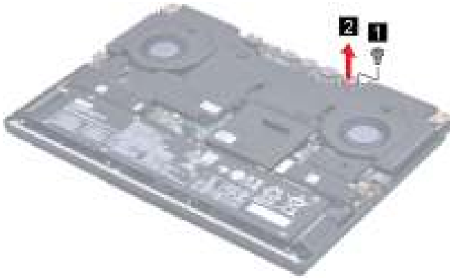
Figure 21. Remove the DC-in bracket
