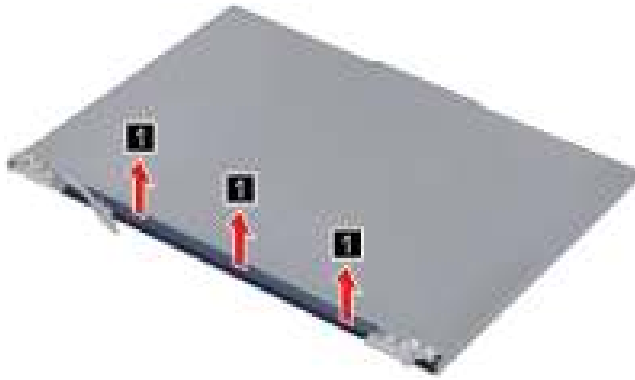
Figure 59. Remove the hinge cover
