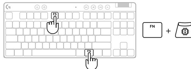
**2** Start justeringstilstand for Hurtig trigger.
